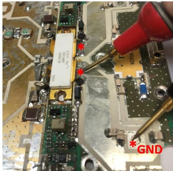
Figure 124: FET resistance test
