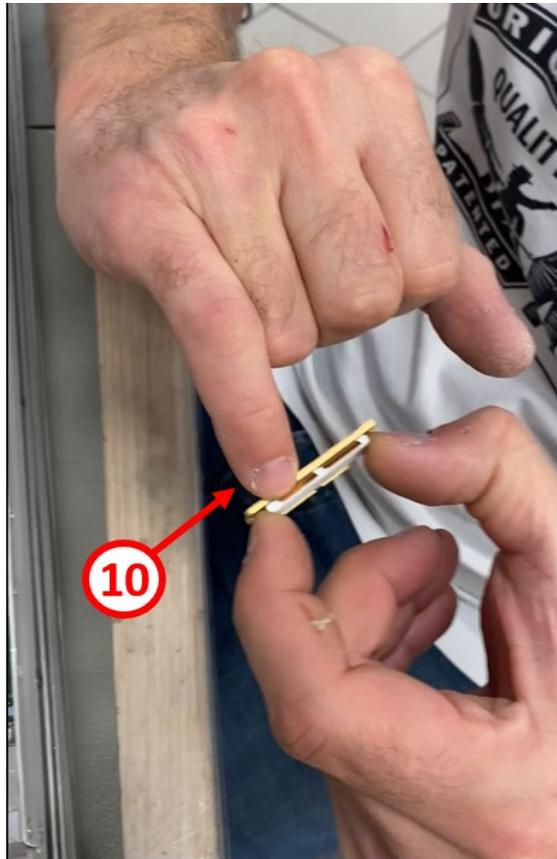
Figure 136: Remove excess thermal grease
