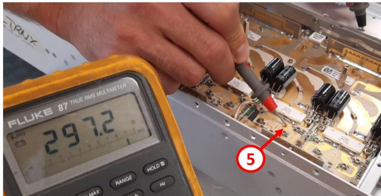
Figure 130: FET resistance test, right gate tab
