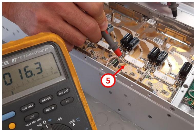
Figure 129: FET resistance test, left gate tab
