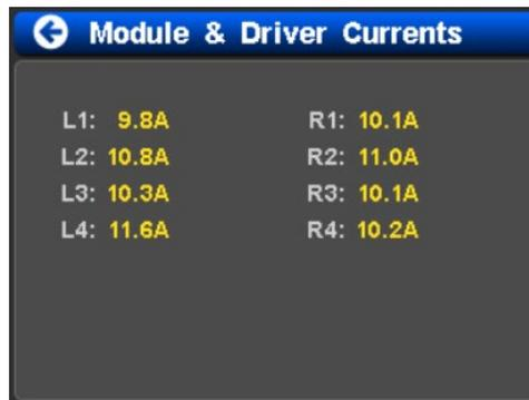
Figure 55: LCD Home > Main Menu > Amplifier > PSU Status > Currents menu
