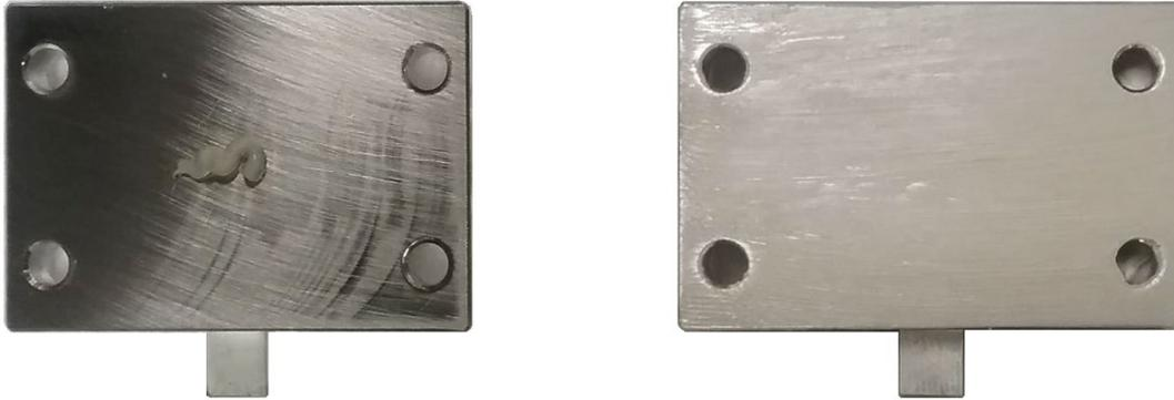
Figure 145: Spread thermal compound on mounting flange
