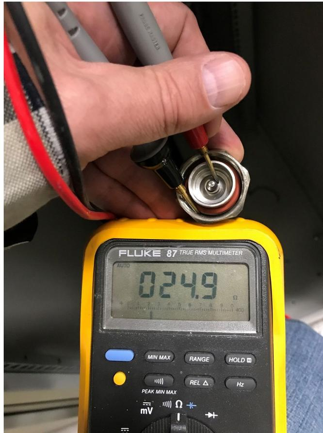
**Figure 142: Measure load port resistance**
