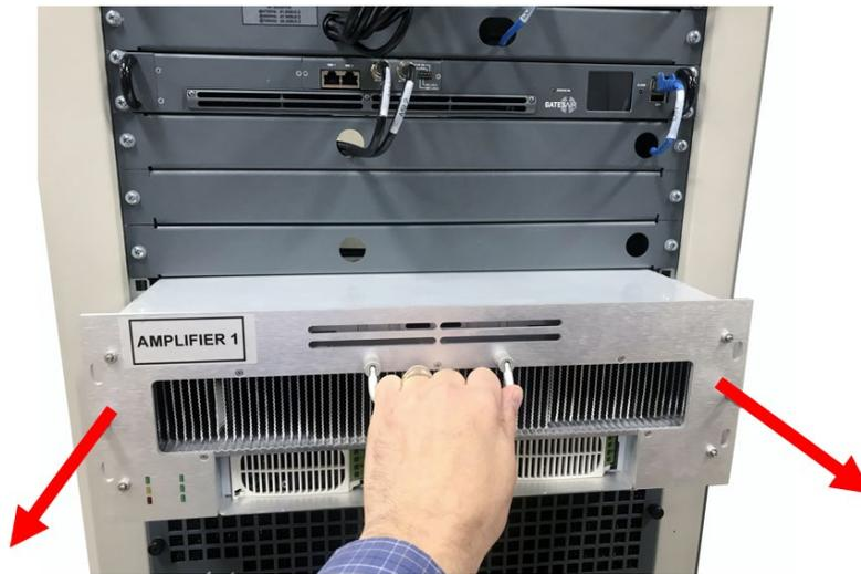
Figure 119: Extracting the amplifier
