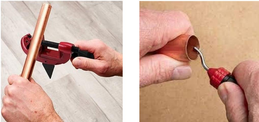
Figure 10: Cut and deburr transmission line
