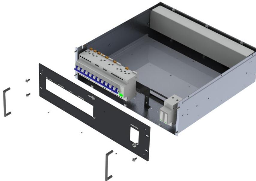
Figure 146: Remove front panel
