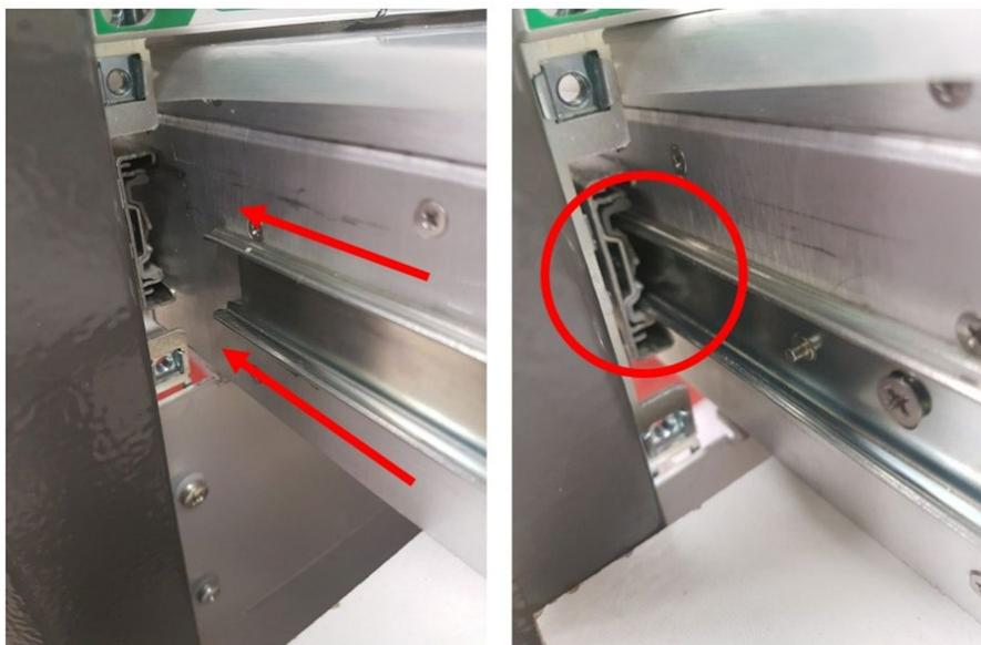
Figure 7: Sliding guides check
